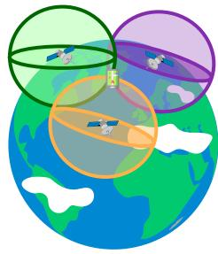
When calculating 3D position, we need 3 satellites to work out the X Y Z position of our receiver, but the receiver clock is poor compared to the atomic clock in the satellite. As the whole system is based on time, one more satellite is needed to determine the receiver clock bias, therefore we need at least 4 satellites.
